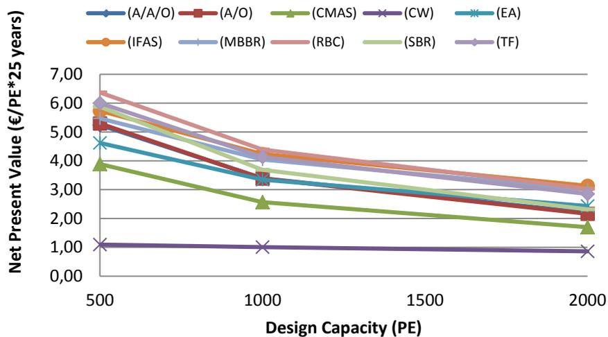
Figure 2. Net present value for high loading and average discharge limits.
