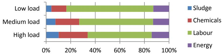
Figure 3. Effect of variation in load on the percentage contribution of OPEX components for MBBR systems
