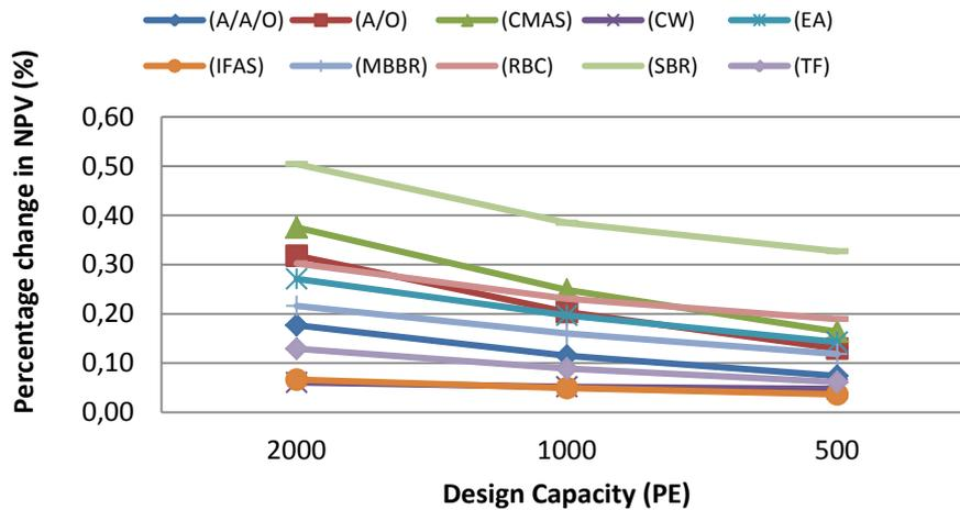
Figure 1. Percentage change in NPV from high to low organic loading with medium level discharge limits.
